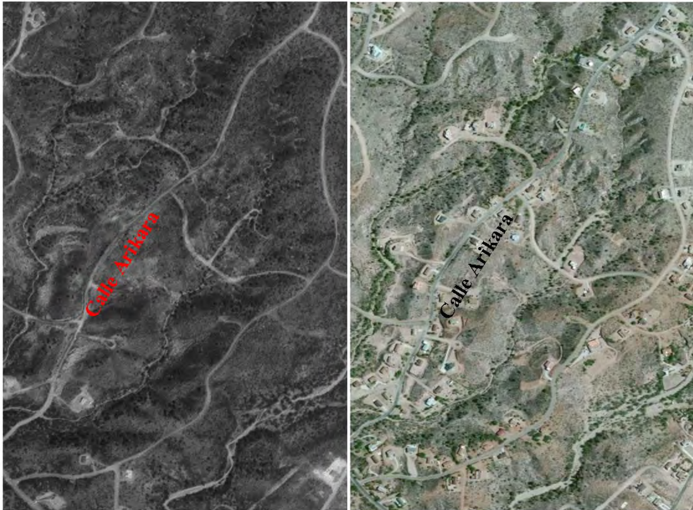
Figure 1: Aerial photography of Calle Arikara road in Rio Rico from 1992 (left) and 2010 (right) confirming chip-seal paving of the roadway occurred between these dates.
