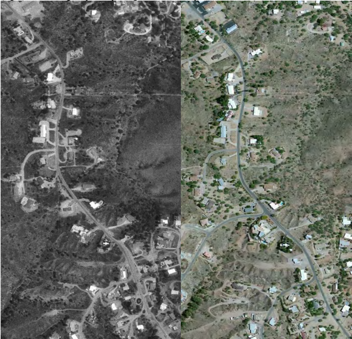
Figure 6: Aerial photography of Royal Road in Nogales from 1992 (left) and 2010 (right) confirming chip-seal paving of the roadway occurred between these dates.
