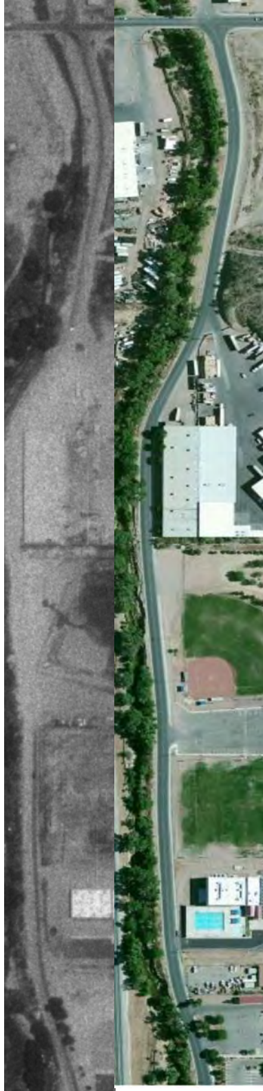
Figure 7: Aerial photography of Hohokam Road in Nogales from 1992 (left) and 2010 (right) confirming chip-seal paving of the roadway occurred between these dates.
