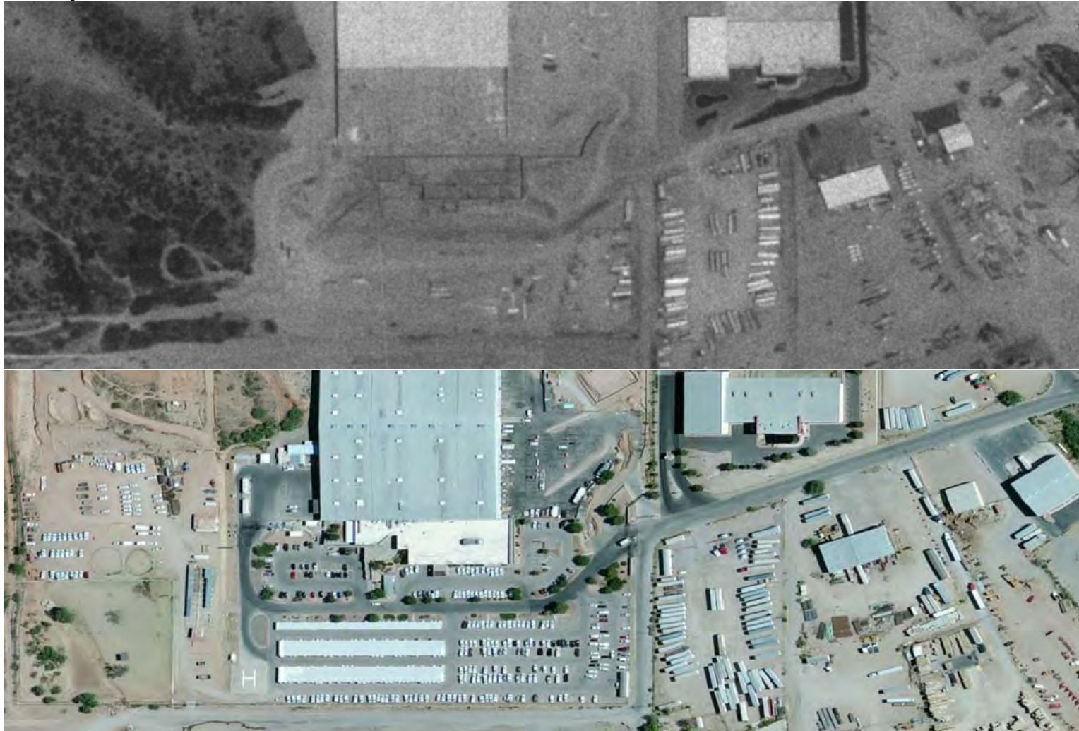
Figure 8: Aerial photography of La Quinta Road in Nogales from 1992 (top) and 2010 (bottom) confirming chip-seal paving of the roadway occurred between these dates.
