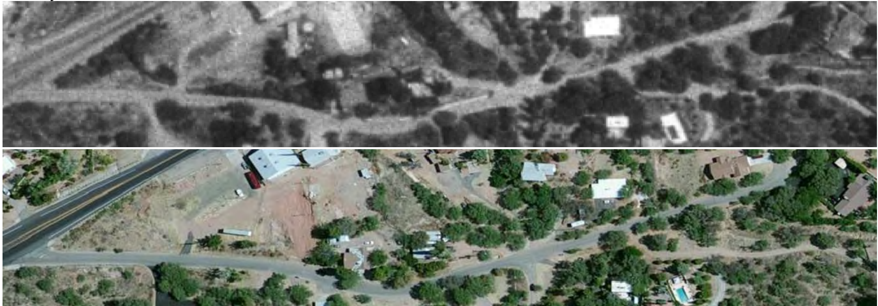
Figure 10: Aerial photography of Bristol Dr. in Nogales from 1992 (top) and 2010 (bottom) confirming chip-seal paving of the roadway occurred between these dates.
