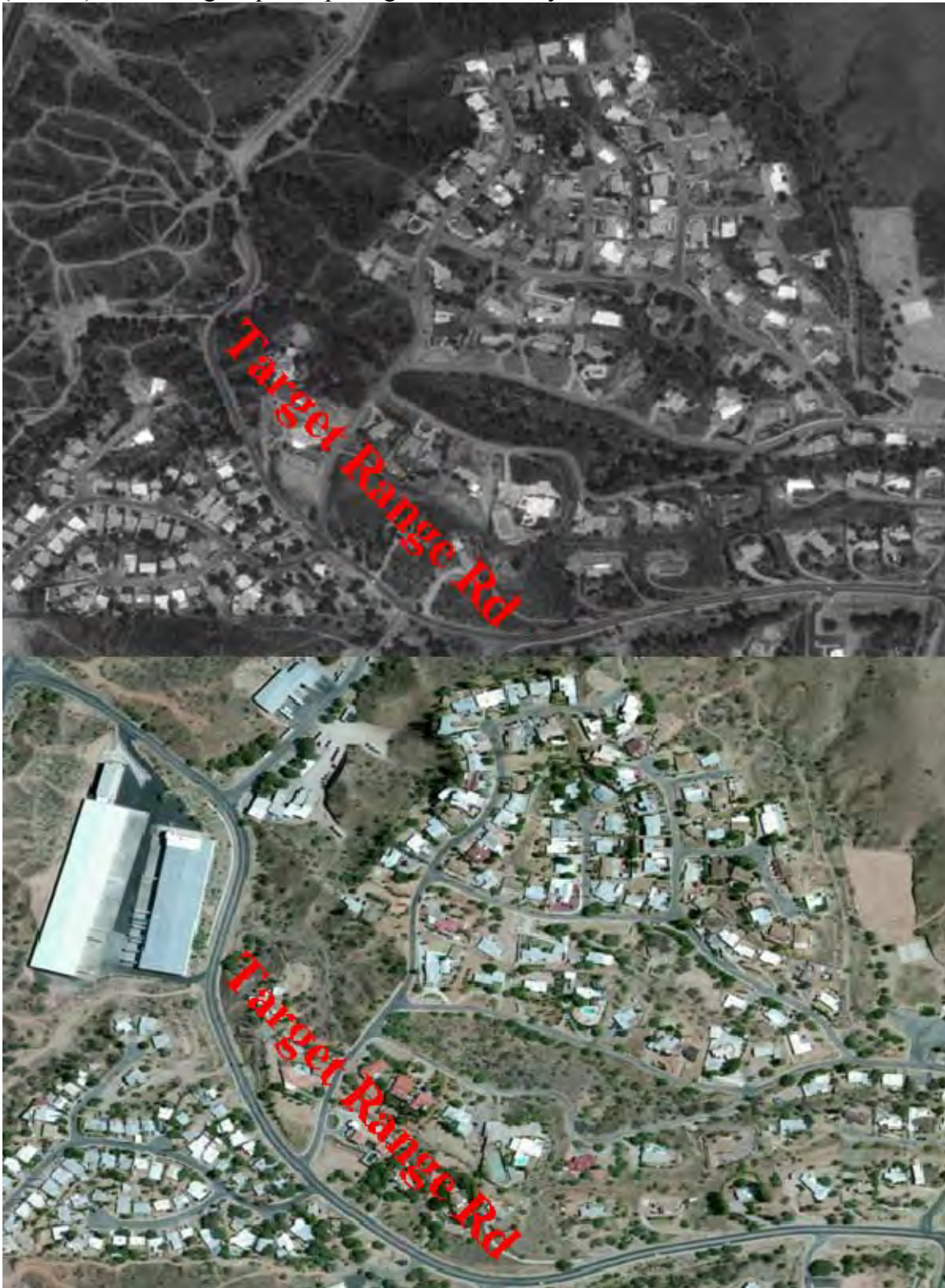
Figure 11: Aerial photography of Target Range Rd. in Nogales from 1992 (top) and 2010 (bottom) confirming chip-seal paving of the roadway occurred between these dates.
