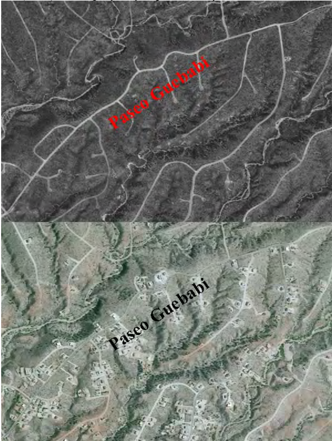
Figure 5: Aerial photography of Paseo Guebabi road in Rio Rico from 1992 (top) and 2010 (bottom) confirming chip-seal paving of the roadway occurred between these dates.
