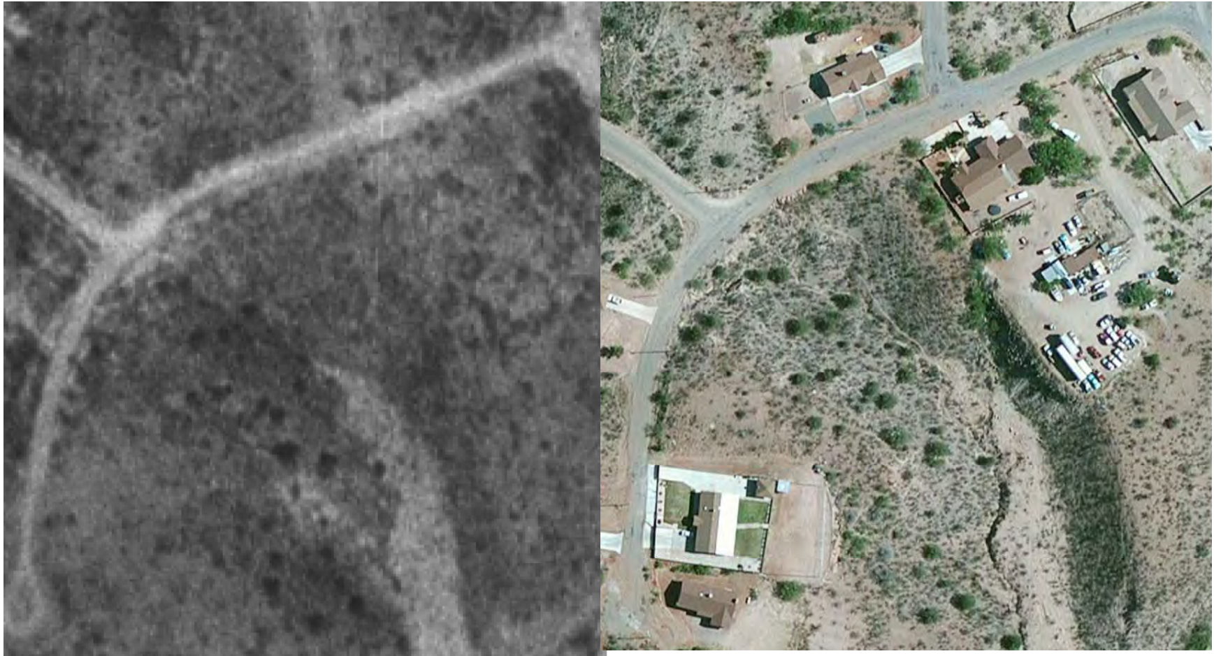
Figure 4: Aerial photography of Annette Ct. in Rio Rico from 1992 (left) and 2010 (right) confirming chip-seal paving of the roadway occurred between these dates.
