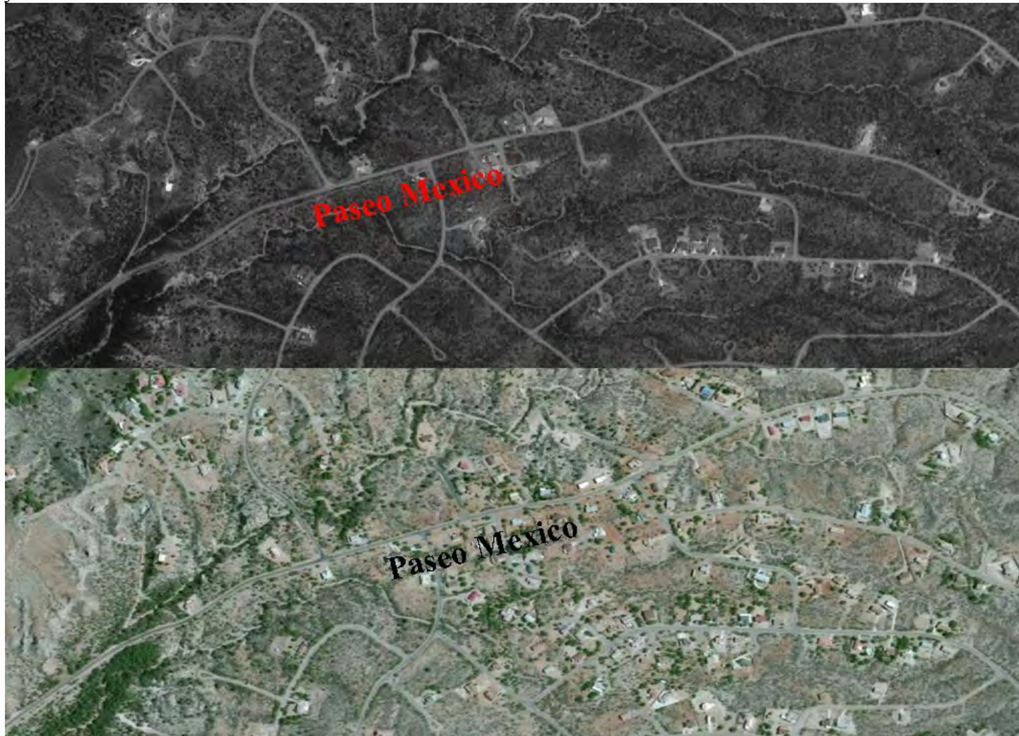
Figure 2: Aerial photography of Paseo Mexico road in Rio Rico from 1992 (top) and 2010 (bottom) confirming chip-seal paving of the roadway occurred between these dates.
