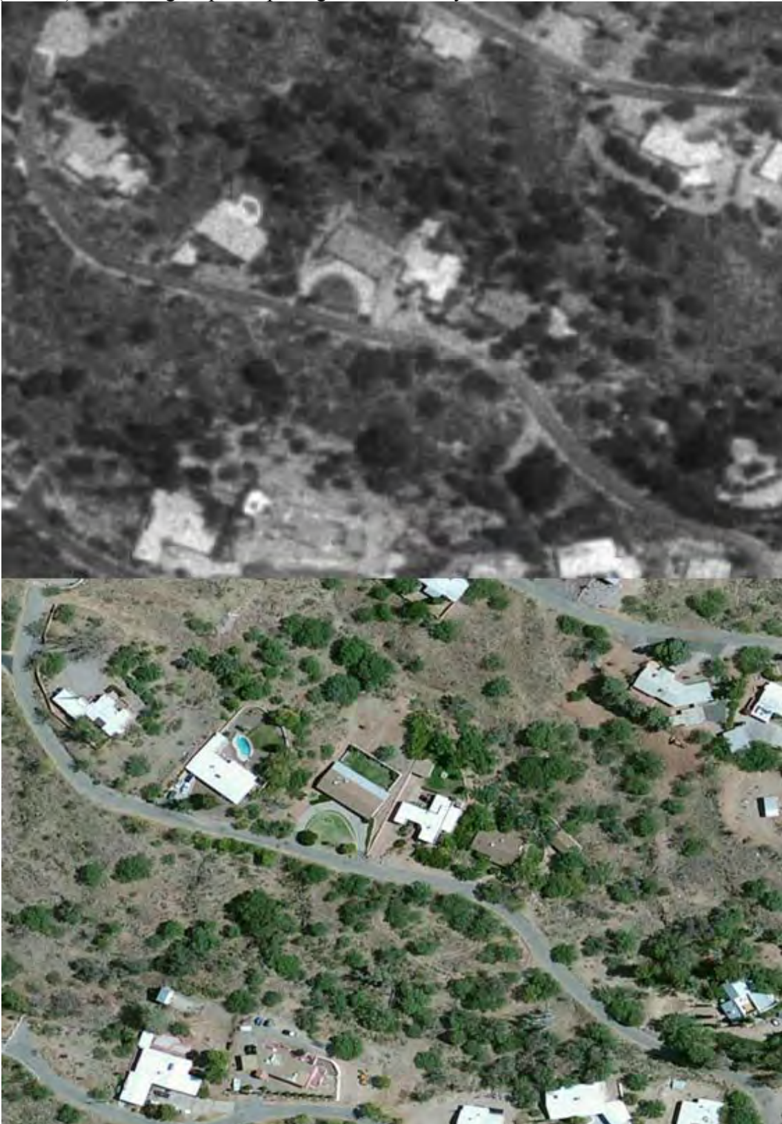
Figure 9: Aerial photography of Yucca Dr. in Nogales from 1992 (top) and 2010 (bottom) confirming chip-seal paving of the roadway occurred between these dates.
