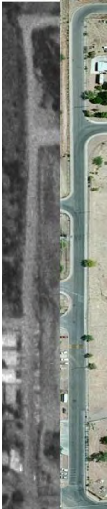
Figure 14: Aerial photography of Kelsey Ave. in Nogales from 1992 (top) and 2010 (bottom) confirming chip-seal paving of the roadway occurred between these dates.
