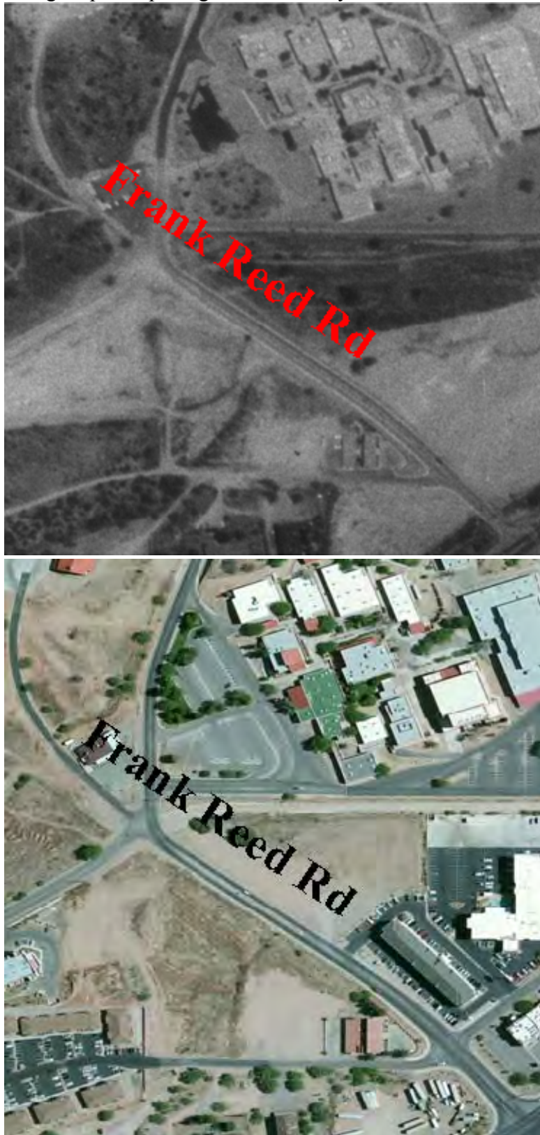
Figure 12: Aerial photography of Frank Reed Rd. in Nogales from 1992 (top) and 2010 (bottom) confirming chip-seal paving of the roadway occurred between these dates.
